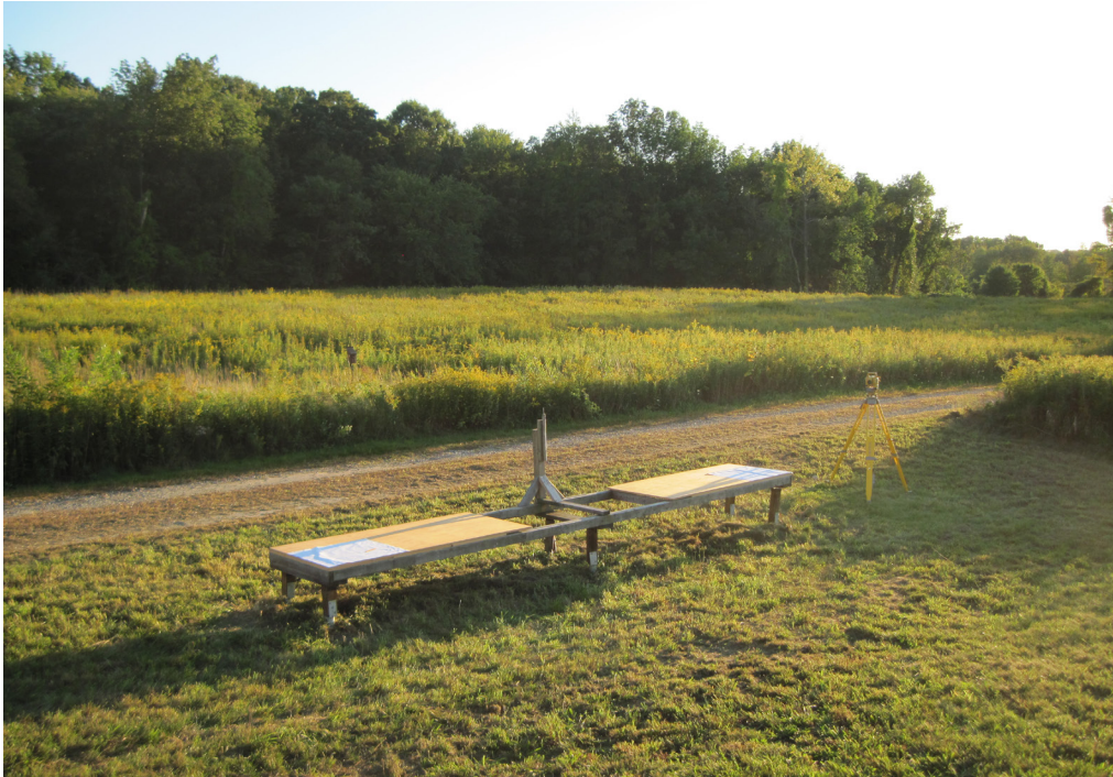
Fig. 3. The equinoctial solar gnomon method was tested on this platform, here viewed from the northeast. In the center of the platform is the gnomon, set along its midline on its southern edge.
