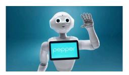
Pepper is humanoid and programmable robot and its height is 120 centimeters. Its design oriented to interact with people, has a technology that allows to analyze verbal and non-verbal language, head position and voice tone.
