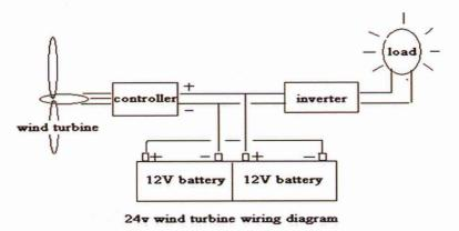
if you choose the 12v wind turbine, you need to use the 12v battery, 12v controller, 12v inverter, you can use the battery quantity based on your actual needs, for more than 2pcs you can use parallel connection.
