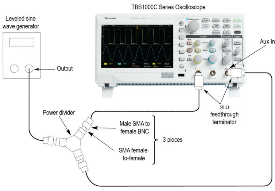
3. Set the oscilloscope **Vertical Scale** (volts/division) to **100 mV/div**.
