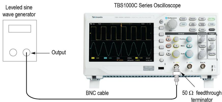
3. Set the oscilloscope **Vertical Scale** (volts/division) to **500 mV/div**.
