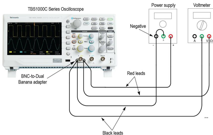
4. Set the power supply to the 1.8 V value shown in column A, the Approximate Test Voltage.
