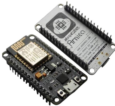
*Ilustración 2. NodeMCU V2 Amica. Fuente: <https://www.electronicwings.com/nodemcu/nodemcu-development-kitboard>*
