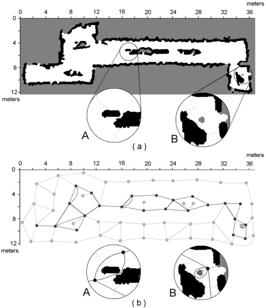
**Fig. 3.** a) Thresholded global grid-map of an office-like indoor environment (white-free space; black- obstacles and grey- non-explored); and b) highest level of the hierarchy of dual graph which encodes the topological representation (black nodes- free space and grey nodes- non-explored)
