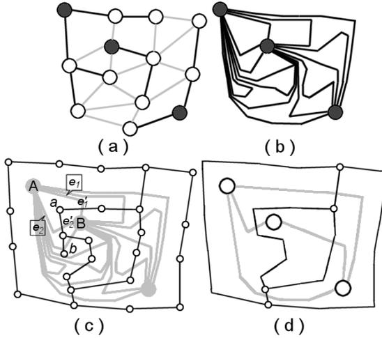
**Fig. 2.** Contraction and removal kernels: a) contraction kernel composed of three vertices (surviving vertices are marked in black); b) reduction performed by the equivalent contraction kernel in a); c) redundant edges characterization; and d) dual graph pair  $(G, \tilde{G})$  after dual decimation step
