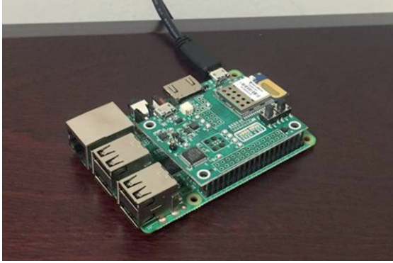
Fig. 5. Smart accurate beacon composed of Raspberry pi 3 with UWB technology.
