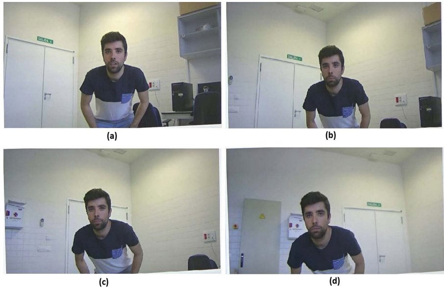
Fig. 11. Experiments. The figures depict the images of the monitor screen (a)–(d) The speaker is moving towards his right side, and the camera corrects its orientation in order to center his face
