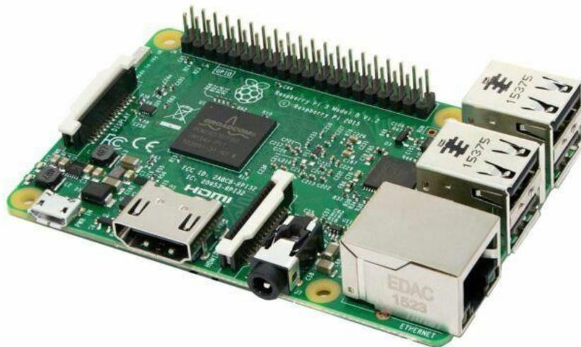
*Figura 13. Raspberry Pi 3 Model B.*
