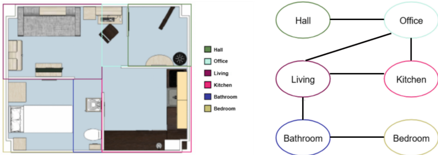
Fig. 4. On the left, a plan of the experimental environment divided into six distinct locations. On the right, undirected graph representing the physically possible transitions between locations.
